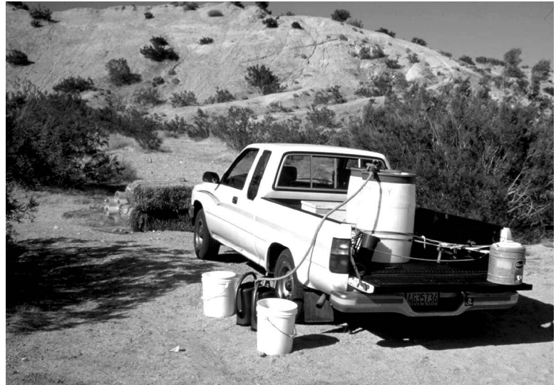
Figure 2. A typical arid land water setup using 30-gallon drums and hoses. No pump is required, all water delivery is gravity-fed. Drums must be securely fastened to the bed of the pickup.
