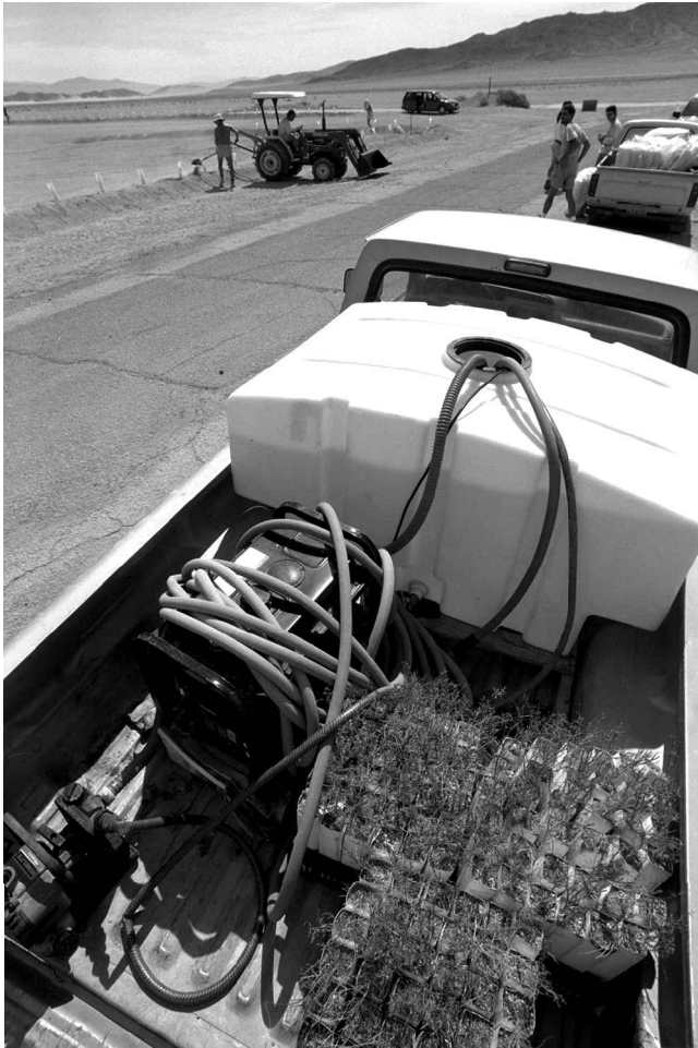
Figure 1. A water truck with a motorized pump and multiple hoses stands ready to water seedlings. Photos and illustrations courtesy of David A. Bainbridge
